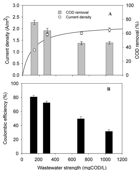
**Figure 2.** Relationship between initial DWW strength with COD removal and produced current density (A) and CE (B) in the thermophilic MFC with a cathode of one Pt-coated sheet.
