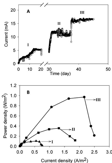
**Figure 1.** Current (A) and power (B) production from thermophilic MFC operated with DWW at different cathode electrode conditions (bare (I), one Pt-coated sheet (II), and two Pt-coated sheets (III)).
