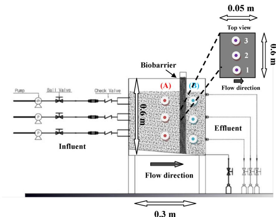
**Fig. 1.** Schematic presentation of the bench-scale set-up horizontally. Note: Three sampling points at positions (A) and (B) represent the diesel analysis at the left/right of the biobarrier. Three sampling points of position (1–3 points) in the biobarrier represent microbiological analysis.
