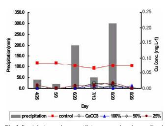
Fig. 3. Precipitation and copper (Cu) concentrations in runoff and leachate. The % numbers indicate the amount of lime cake as % LR.
