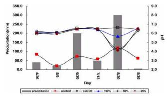
Fig. 2. Precipitation and pH in run-off and leachate.
