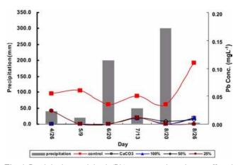
Fig. 4. Precipitation and lead (Pb) concentrations in runoff and leachate. The % numbers indicate the amount of lime cake as % LR.
