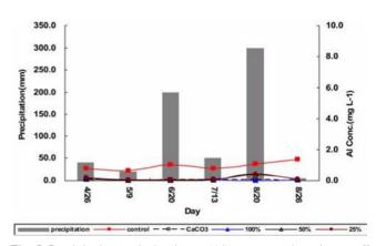
Fig. 5. Precipitation and aluminum (Al) concentrations in runoff and leachate. The % numbers indicate the amount of lime cake as % LR.
