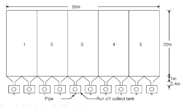
Fig. 1. Cross section (bird eye's view) of the field experimental system.
