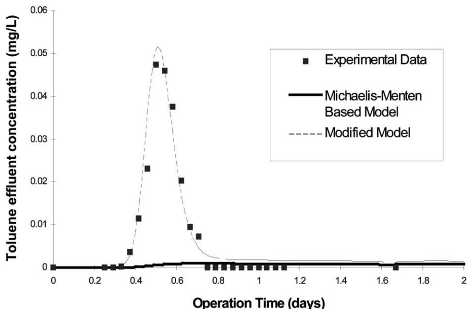
Fig. 5. Comparison of different model simulations with the first toluene breakthrough curve (peak A in Fig. 2) observed in the column experiment.
