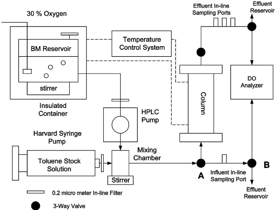
Fig. 1. Column apparatus schematic. The temperature of the basal salts medium (BM) reservoir and column was controlled at  $25 \pm 0.5^\circ\text{C}$ .
