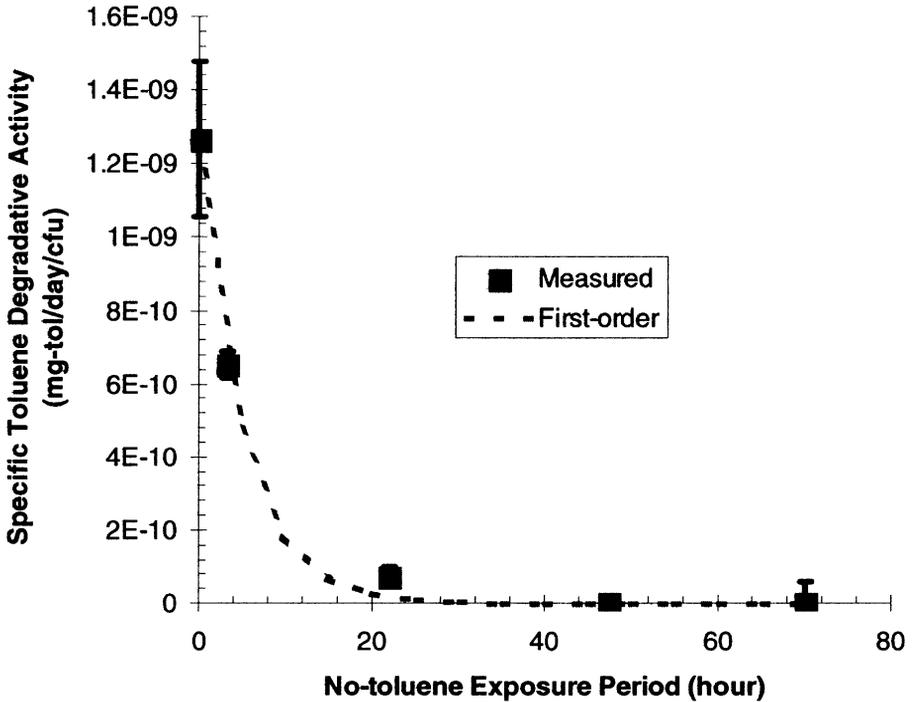
Fig. 6. Specific toluene degradative activity (initial toluene concentration = 1.4 mg/l) versus no-toluene exposure period. Each filled square represents the average value, and the Y-error bar represents one standard error of the average value.
