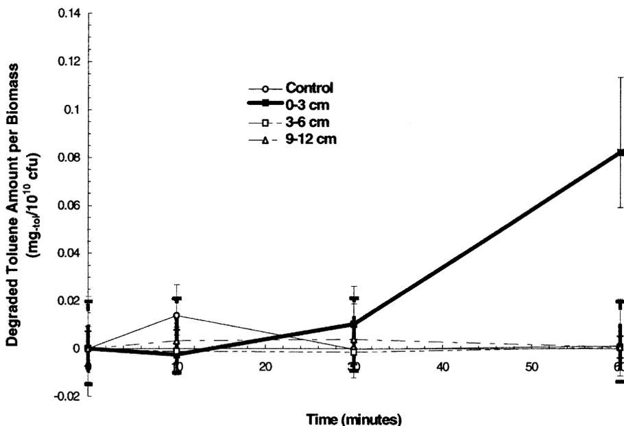
Fig. 3. Biomass normalized toluene degradation (initial toluene concentration = 0.3 mg/l) in cells extracted from column core samples at the end of column experiment. The numbers in the annotation indicate distance from the column inlet. The uncertainty in biomass quantification and the differences between duplicate degradation measurements were incorporated into the calculation of the Y-error bars.
