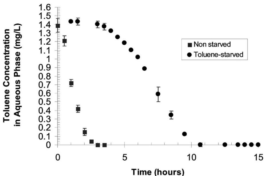
Fig. 7. Toluene (aqueous phase) concentration versus time in the toluene degradation batch experiments with nonstarved and toluene-starved PKO1 cells (suspended growth). The filled squares and the filled circles represent the average values, and the Y-error bar represents one standard error of each average value.
