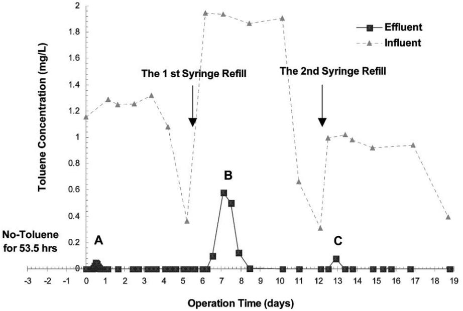
Fig. 2. Influent and effluent toluene concentrations in the column experiment. The measured hydraulic retention time was  $11.6 \pm 0.1$  h.
