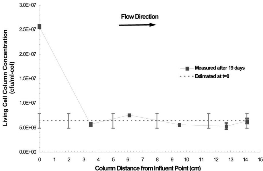
Fig. 4. Spatial distributions of living cell concentrations before and after the column experiment. The filled squares and the dashed line represent the average values. The Y-error bar represents one standard error of the measured average value.
