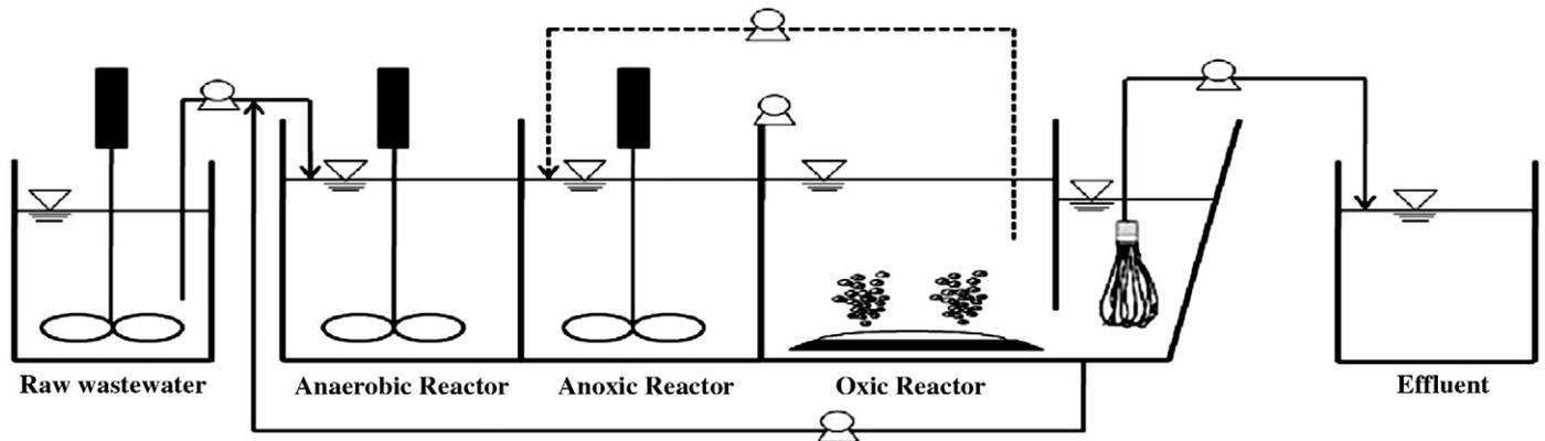
Fig. 1. Schematic diagram of membrane bioreactor system.
