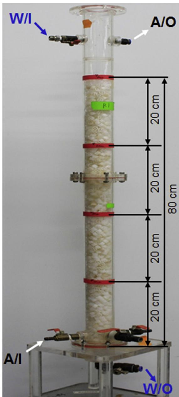
Fig. 2. Stripping column packed with polyethylene carriers. Four ports were installed on the column for water inlet (W/I), water outlet (W/O), air inlet (A/I), and air outlet (A/O).
