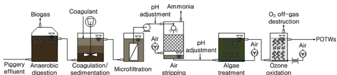
**Fig. 1.** Schematic of integrated strategies for robust treatment of high saline piggery wastewater.
