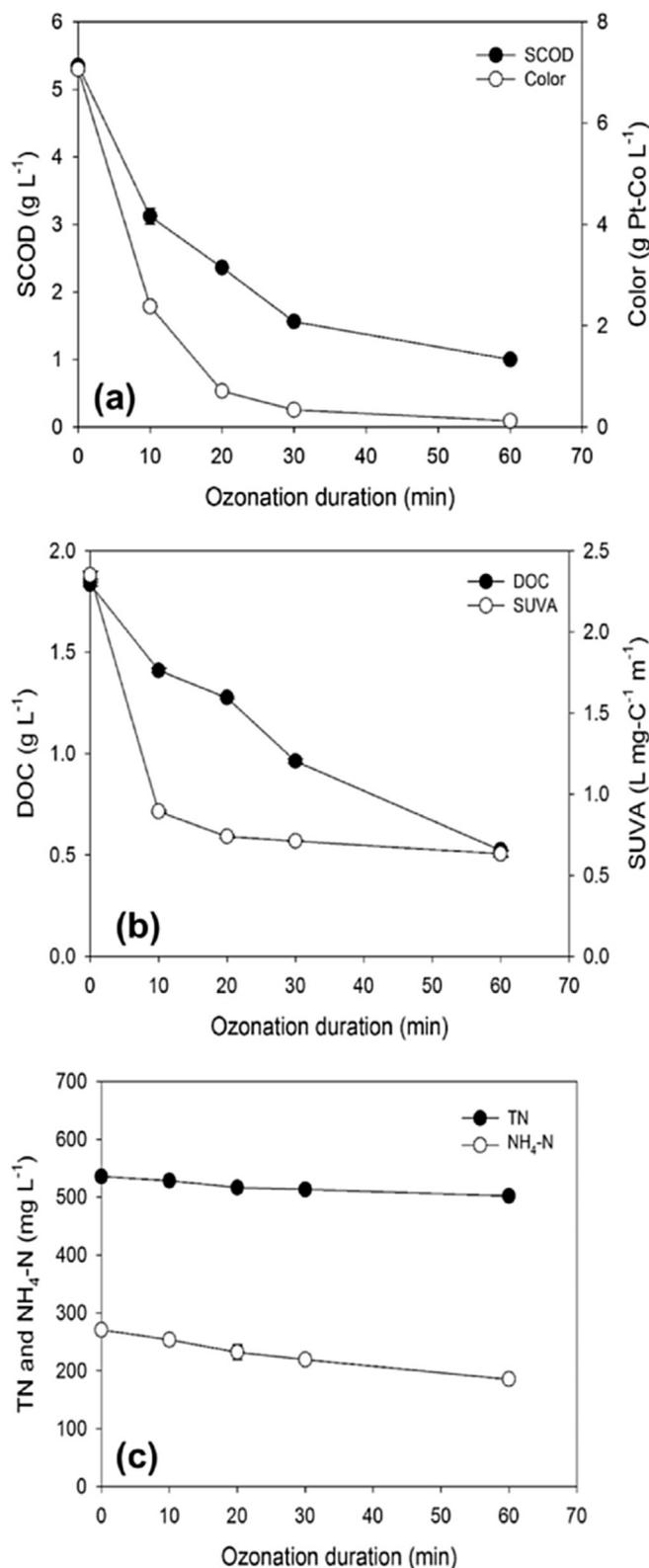
Fig. 4. Impact of ozonation on the characteristics of piggery wastewater. The ozonation of piggery wastewater continued up to 60 min at a dose of 87 mg O<sub>3</sub> L<sup>-1</sup>.
