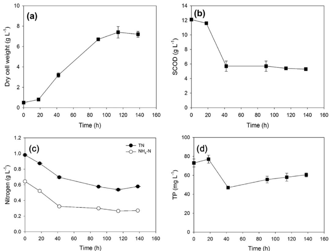
Fig. 3. Growth of *S. quadricauda* and the associated removal of contaminants. The residual concentrations of COD, TN, NH<sub>4</sub>-N, and TP were determined after filtration (0.2 μm).
