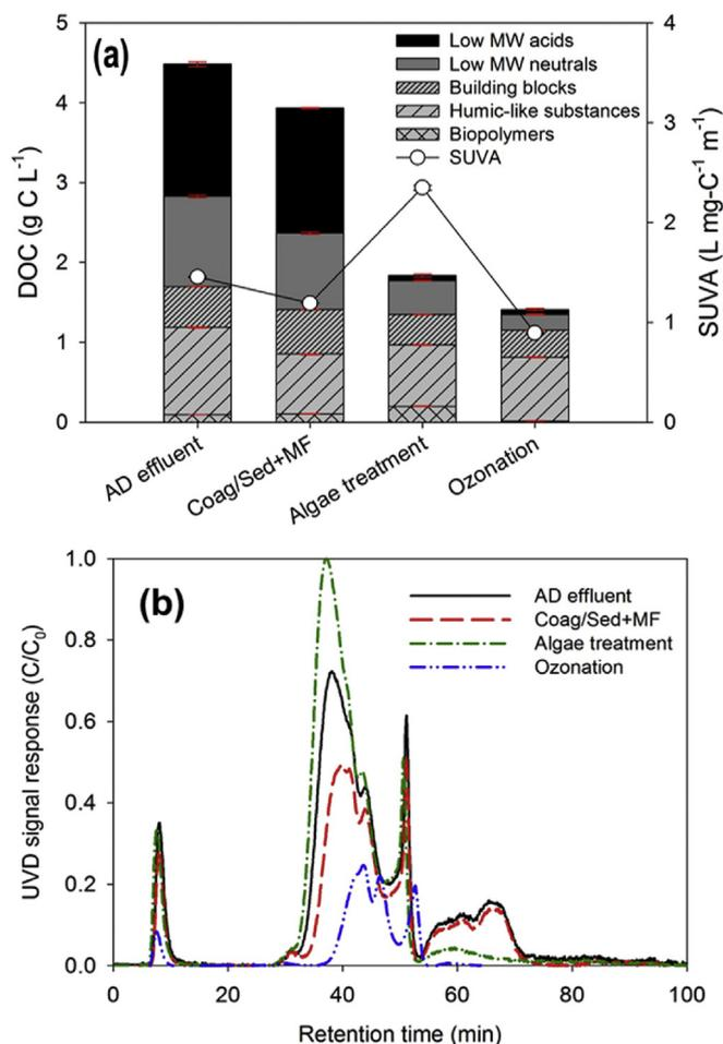
**Fig. 5.** (a) Effects of sequential treatments on the distributions of five different organic fractions in piggery effluent. (b) LC-UV-Vis spectra for organic materials in the piggery wastewater samples. Ozonation was 10 min at a dose of 87 mg O<sub>3</sub> L<sup>-1</sup>.
