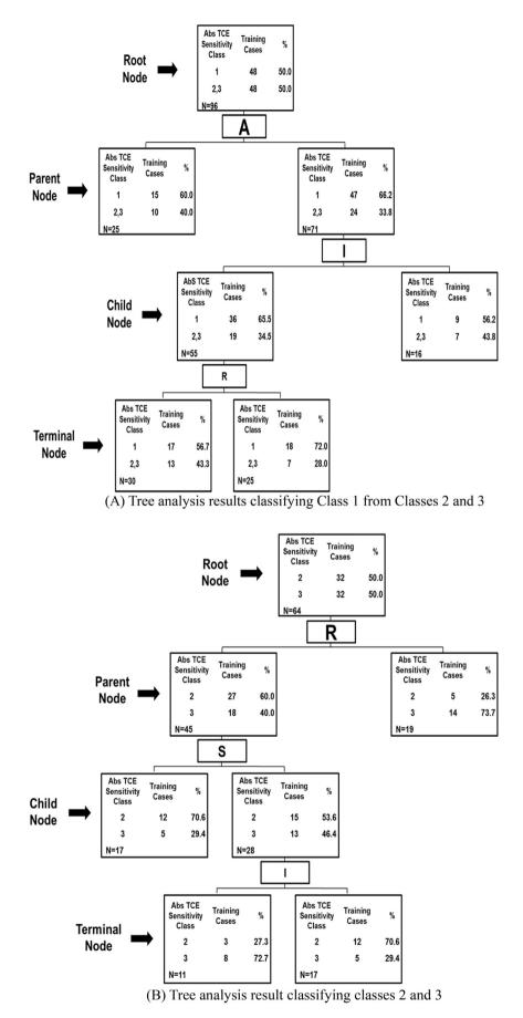
**Fig. 5.** One example of a CART based tree analysis result. Each node is labeled with each class, training cases, and the number (N) of data samples in that group. The model is read from top down until terminal nodes appear. Influential variables are presented in parentheses at each root node to split. (A) indicates the result classifying class 1 from the others, and (B) indicates the result classifying classes 2 and class 3.
