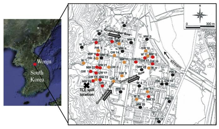
Fig. 6. The distribution of groundwater TCE sensitivity in Woosan Industrial Complex. Red points indicate high TCE sensitivity wells (TCE sensitivity 3), Orange points indicates medium TCE sensitivity wells (TCE sensitivity 2), and Black points indicate low TCE sensitivity wells (TCE sensitivity 1). (For interpretation of the references to colour in this figure legend, the reader is referred to the web version of this article.)
