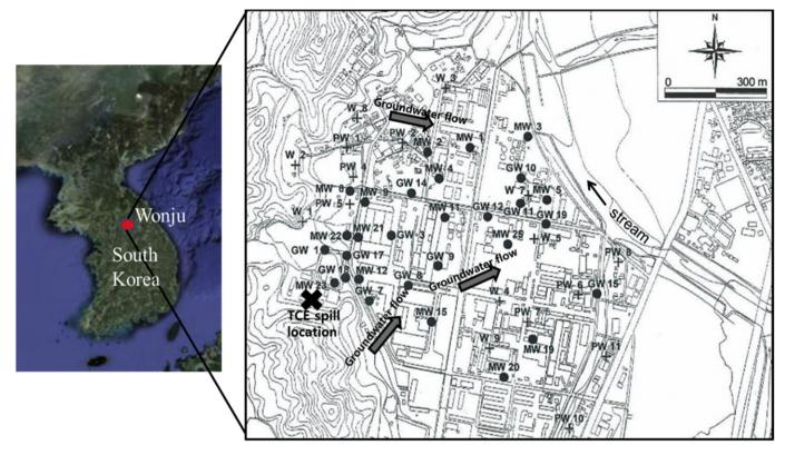
Fig. 1. Location of the Woosan Industrial Complex area. The groundwater wells at the study site are shown. The TCE spill location, which is regarded as the primary source of TCE contamination, is also shown by (X).
