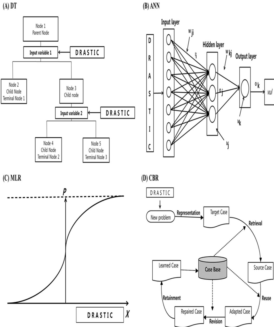
Fig. 3. Conceptual schemes of the data mining methods used in this study: the structure of CART process in DT (A), ANN process (B), MLR process (C), and CBR process (D).
