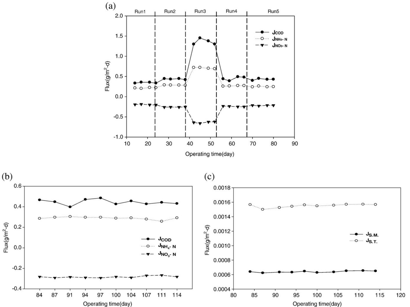
Fig. 5. Results of  $J_{COD}$ ,  $J_{NH_4^+-N}$ ,  $J_{NO_3^- -N}$ ,  $J_{S.M.}$ , and  $J_{S.T.}$  according to experimental conditions. (a)  $J_{COD}$ ,  $J_{NH_4^+-N}$ , and  $J_{NO_3^- -N}$  without sulfamethazine and sulfathiazole. (b)  $J_{COD}$ ,  $J_{NH_4^+-N}$ , and  $J_{NO_3^- -N}$  including sulfamethazine and sulfathiazole. (c)  $J_{S.M.}$  and  $J_{S.T.}$ .
