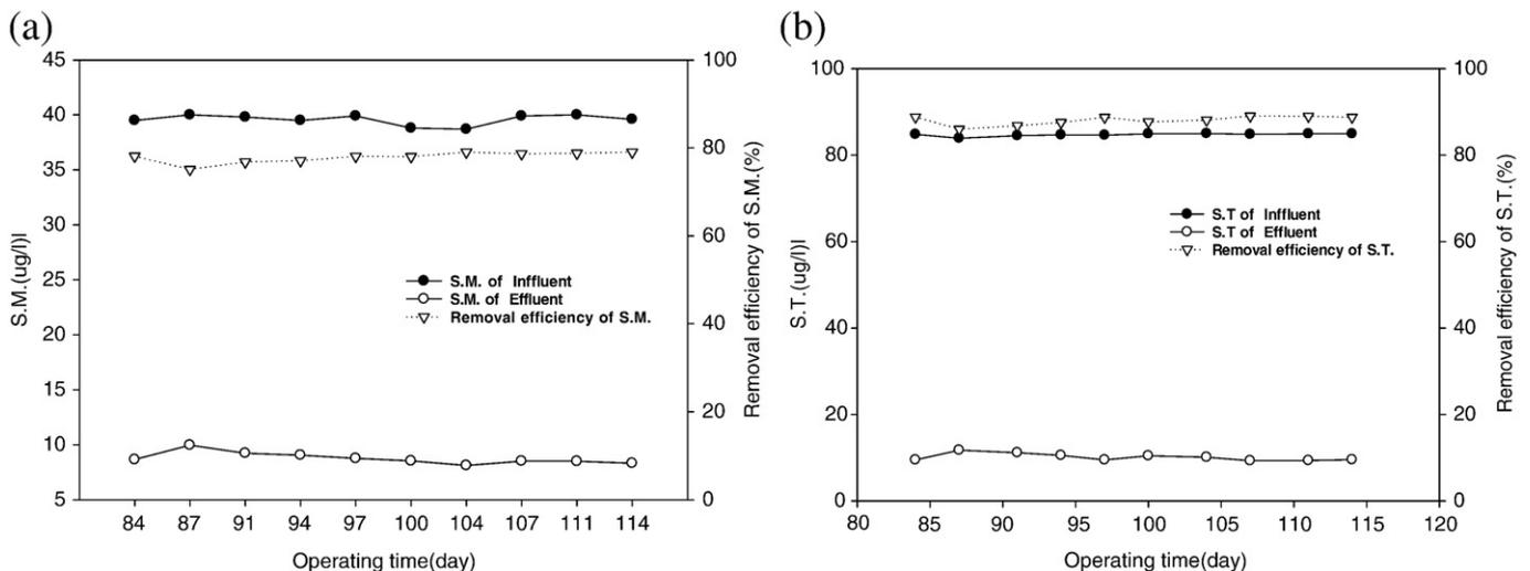
**Fig. 3.** Experimental results of sulfamethazine (S.M.) and sulfathiazole (S.T.). (a) Concentrations and removal efficiency of sulfamethazine in set II experiment. (b) Concentrations and removal efficiency of sulfathiazole in set II experiment.
