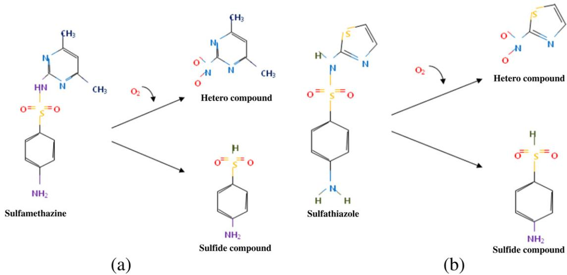
Fig. 4. Expected decomposition pathway of sulfamethazine and sulfathiazole. (a) Pathway of sulfamethazine. (b) Pathway of sulfathiazole.
