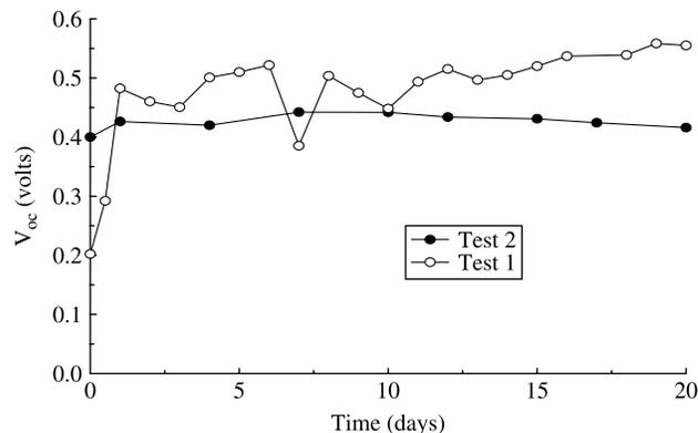
**Figure 1** |  $V_{oc}$  change in response to time. ( $V_{oc}$  = open-circuit voltage. Test 1 indicates that  $V_{oc}$  does not change before biofilm formation, and Test 2 indicates that  $V_{oc}$  changes after biofilm formation).
