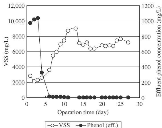
Fig. 3. Reactor biomass (VSS) and effluent phenol concentrations in the high phenol fed MBR.
